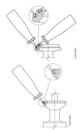
7 Press the seal with your fingers to make sure it is well seated. Make sure there are no parts protruding due to poor positioning of the seal.
